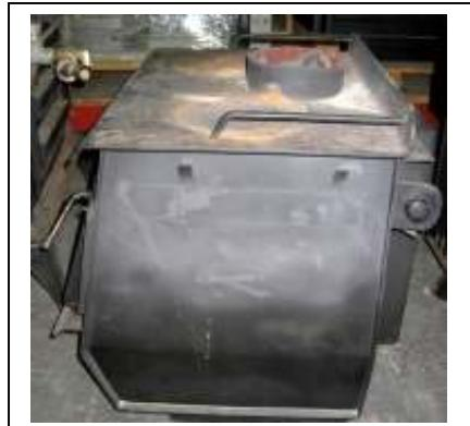
**Construction:** The unit is constructed primarily of mild steel. The firebox is lined with firebrick. The firebox dimensions are: W 16 in x L 13.5 in x H 15.75 in (W 40.6 cm x L 34.3 cm x H 40.0 cm). The feed door has 1.5 in (3.8 cm) braided fiberglass rope gasket.
