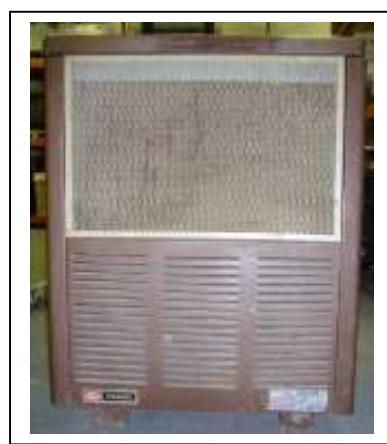
**Construction:** The unit is constructed primarily of mild gauge steel. The firebox is lined with firebrick. The firebox dimensions are: W 11 in x L 17.5 in x H 19.5 in (W 28 cm x L 45 cm x H 50 cm). There is an outer steel shell, with vents, enclosing the unit. The feed door and ash door have 7/8 in (2.2 cm) fiberglass rope gaskets.
