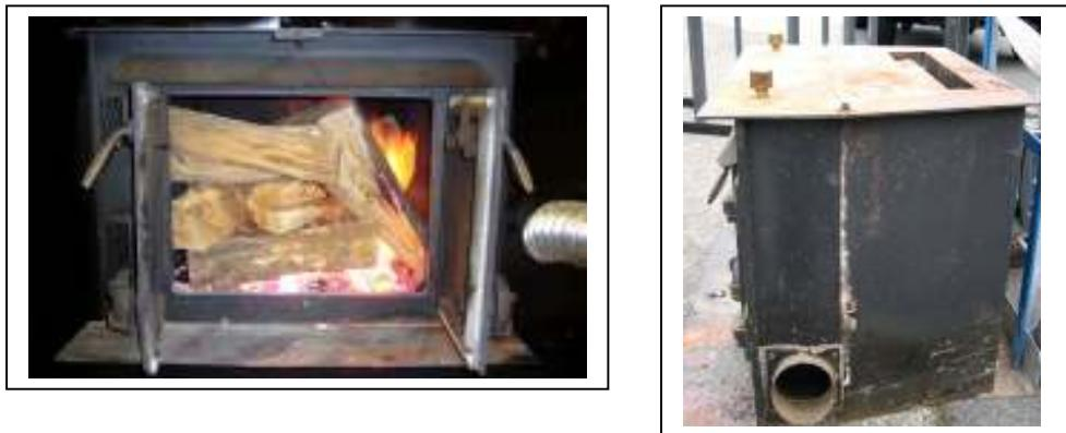
**Construction:** The unit is constructed primarily of heavy gauge steel. The firebox has a cement base. The firebox dimensions are: W 22 in x L 14.9 in x H 17.5 in (W 50.8 cm x L 37.8 cm x H 47.0 cm). The firebox is surrounded by an air circulation area. The feed doors are cast iron and have two ½ in (1.3 cm) flat braided fiberglass gaskets.
