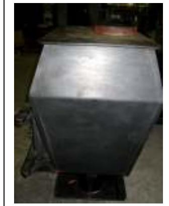
**Construction:** The unit is constructed primarily of steel. The firebox is lined with firebricks. The firebox dimensions are: W 19 in x L 22.5 in H x22 in (W 48.3 cm x L 57.2 cm x 55.9 cm). The doors are aluminum.
