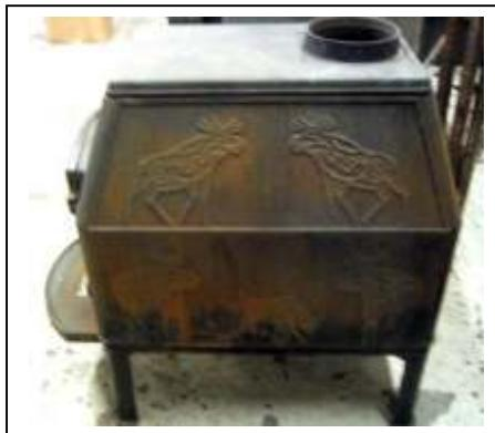
**Construction:** The unit is constructed primarily of cast iron. The unit has a separate cast iron firebox lining. The firebox dimensions are: W 11 in x L 25.5 in x H 15.25 in (W 27.9 cm x L 64.8 cm x H 38.7 cm). The feed door is cast iron with  $\frac{1}{4}$  in (0.625 cm) braided rope gasket.
